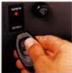
The Toyota Vehicle Intrusion Protection (VIP) RS-3000 System disables the starter and sets off an alarm if a door is opened.
