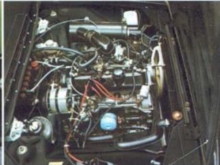
Under the hood...a powerful story! OHV wedgehead engine has a double-chain driven camshaft and double-barrel carburetor.
