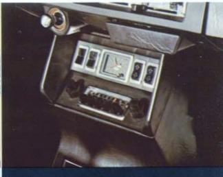
Cockpit control, with electrically-operated windows, 4-speed stick and electric clock all in the console.
