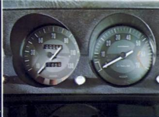
Rally-type instrumentation includes tach and trip recorder, plus a most complete system of gauges and warning lights.
