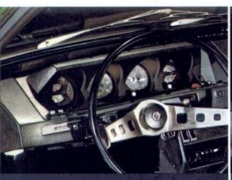
Impressive instrument panel of the Renault 15 includes trip recorder, electric clock, rheostat control for the instrument lighting.
