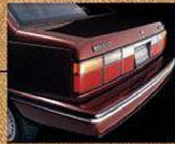
Integral front and rear bumpers contribute to aerodynamics and result in unified styling.
