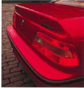
AERODYNAMIC CONTOURING OF THE REAR DECK HELPS REDUCE TURBULENCE BY CONTROLLING THE AIRFLOW AS IT STREAMS OVER AND BEHIND THE LEGEND.
