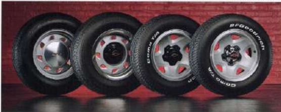
2WD 15" Steel Wheel. Standard on 2WD models. Argent color with bright center cap.
