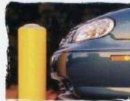
5 MPH Bumpers Malibu's energy-absorbing front and rear bumpers exceed Federal requirements, and feature resilient covers to resist minor dings and dents.
