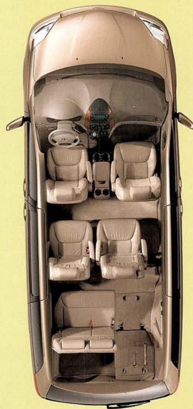
Move the captain's chairs laterally and create cargo room down the side.
