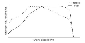
Get the right power curve for your needs. Mack's Maxidyne® engine rating has extended RPM ranges and high torque rise for off-road and jobsite use. MaxiCruise® offers both power and economy for off-road and on-highway.
