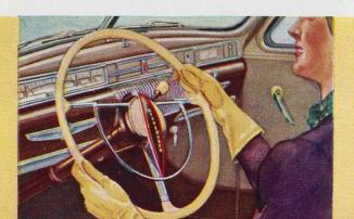
Two-tone phantom wheel with ivory-tone tenite grip and chrome horn ring is standard. Gear shift knob, hardware escutcheons and control knobs are of harmonizing tenite.
