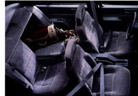
LTZ's luxury interior includes a 60/40 split-folding rear seat that allows access to the trunk.
