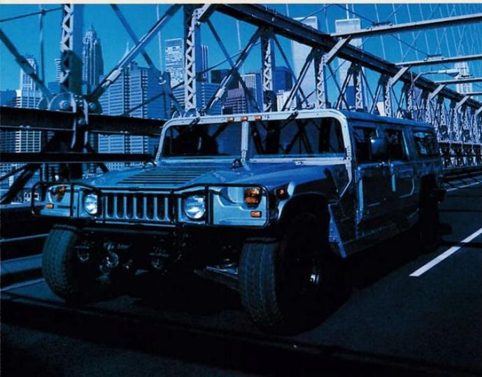
complete with heavy-duty springs and hydraulic shock absorbers. All housed within a seemingly indestructible heat-treated aluminum alloy body. Panels are first bonded together using an epoxy adhesive, then riveted for added strength and durability. It's tough, extremely light, not to mention corrosion resistant. Unrivaled. Uncompromised. Unstoppable.
