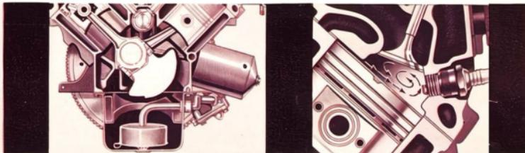
**Deep-block Design** gives far greater rigidity and strength . . . full pressure lubrication system with full-flow oil filtration increases engine life . . . positive-flow crankcase ventilation protects vital parts . . . 3-ring super-fitted, aluminium-alloy pistons give greater efficiency, quietness and life.
