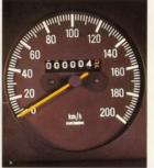
▲ The conventional cable operated speedometer mechanism has been replaced with an electronic pulse system designed to provide improved standards in accuracy and reliability.
