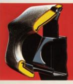
▲ The one-piece, full-foam crash pad and the instrument binnacle are moulded entirely from a special polyurethane foam which is soft inside yet forms its own solid, hard-wearing, easy-care surface.
