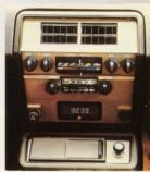
All instrument wiring is channels moulded into the instrument panel. This is designed to improve reliability by greatly reducing the potential for wiring loom pinching and abrasion and the development of squeaks and rattles. The new panel also contains integrated ducts for face-level ventilation and windscreen demisting. Radio available as optional
