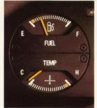
▲ An electronic fuel sender system (similar to those used in Boeing 727 jet aircraft) is designed not only to give more accurate readings of fuel levels. but to provide a more robust system than the mechanically operated device previously used.
