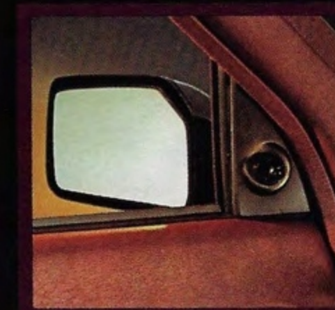
Remote control outside mirror, driver's side.
