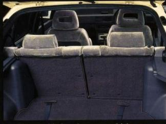
The moulded package tray which normally shields the contents of the rear storage area is easily removed and stored against the back panel, providing added capacity.
