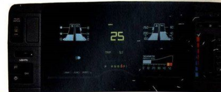
▲ The optional electronic instrument panel provides an easy-to-read cluster: speedometer, tachometer, voltmeter, and gages for fuel, oil pressure and engine coolant temperature.
