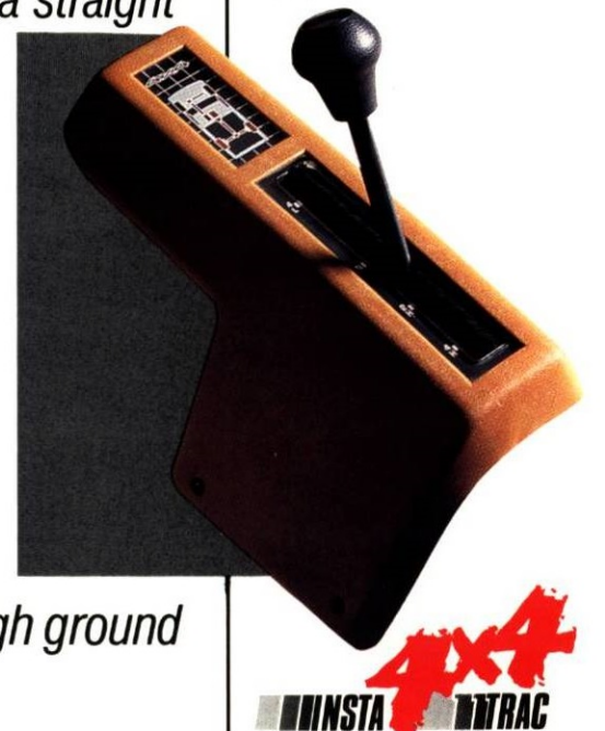
The standard Insta-Trac™ shifter in every 4x4 model is mounted in a lighted console that informs you at a glance of your driving mode. You can shift from 2WD to 4x4 High and back without stopping, at any speed.
