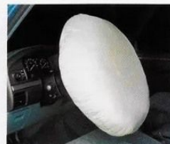
1994 F-Series pickups under 3856 kgs. (8,500-lbs.) GVWR are equipped with a driver-side air bag to supplement the safety belts.
