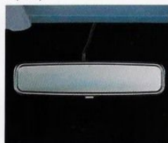
The electrochromic rearview mirror, a new option for the F-Series XLT, automatically dims at night to reduce headlamp glare.
