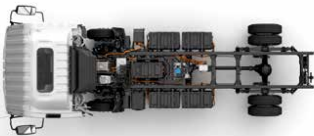
5 Battery Packs - 100 kWh
