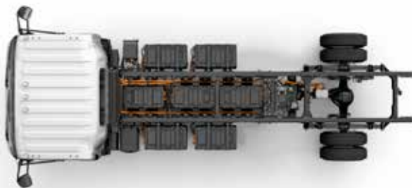
7 Battery Packs - 140 kWh
