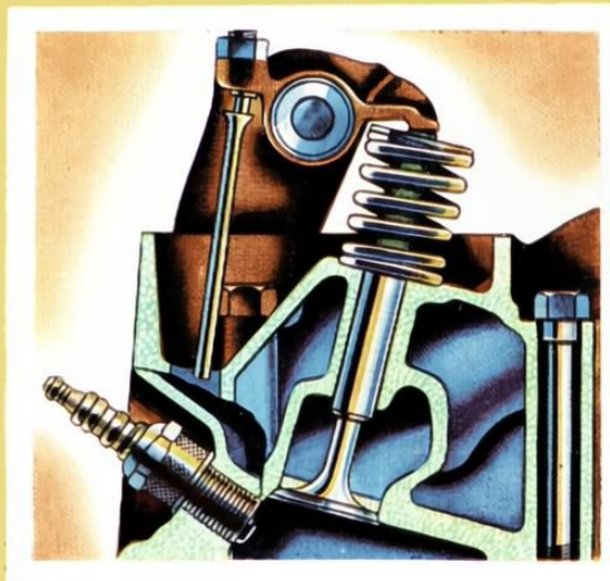
THE OVERHEAD VALVES permit a more efficient combustion head shape which spreads the explosion evenly, giving more power, smoother running and improved fuel consumption.
