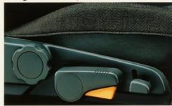
9. In addition to a centre console storage compartment and a trinket tray, Meteor Ghia provides this extremely useful storage tray under the front passenger's seat.
