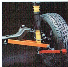
Lumina Sedan's sophisticated technology includes a fully independent suspension and four-wheel power disc brakes.
