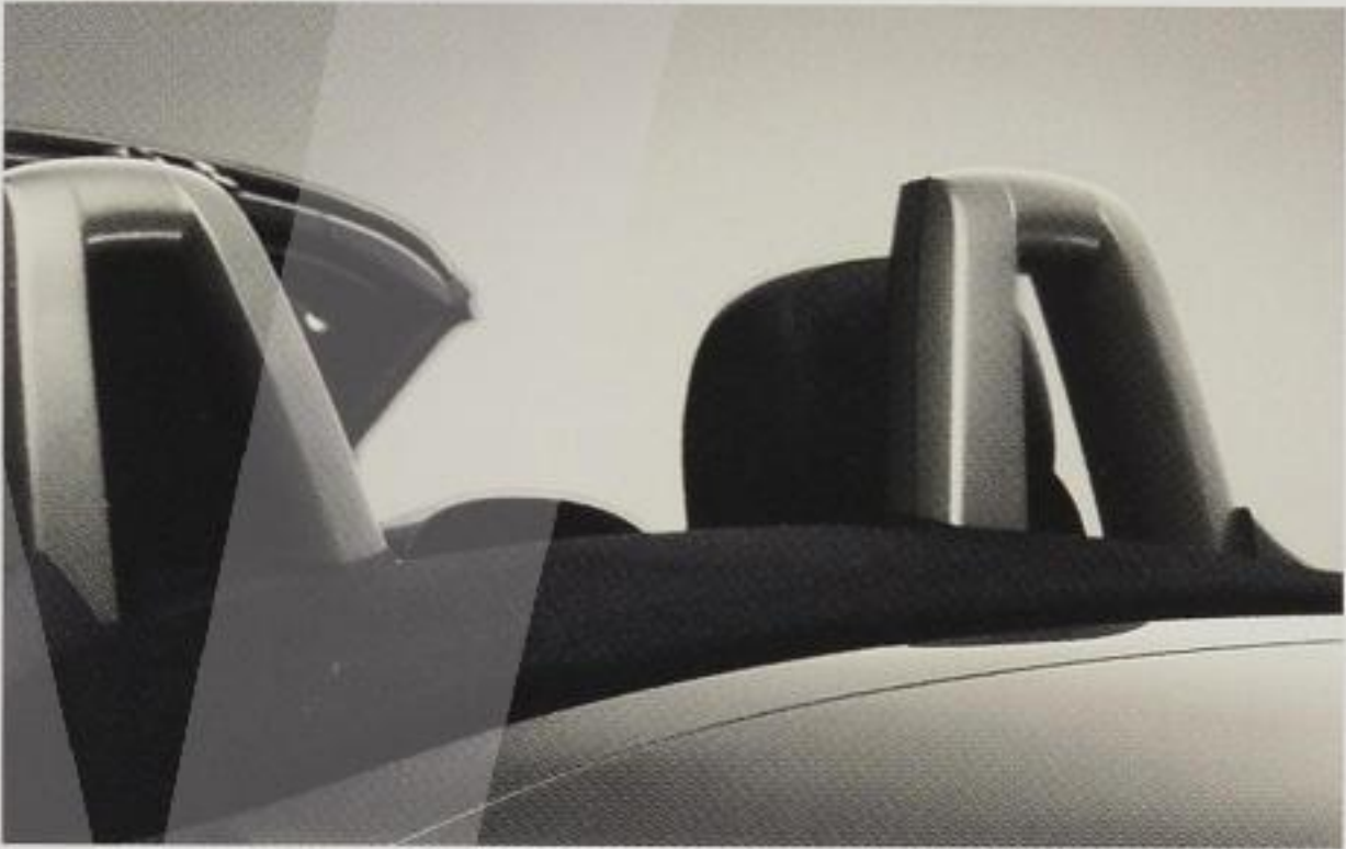
■ Rollover Protection Bars behind the headrests, as well as sheet-tube-reinforced windshield pillars, help provide excellent protection in the event of a rollover.
