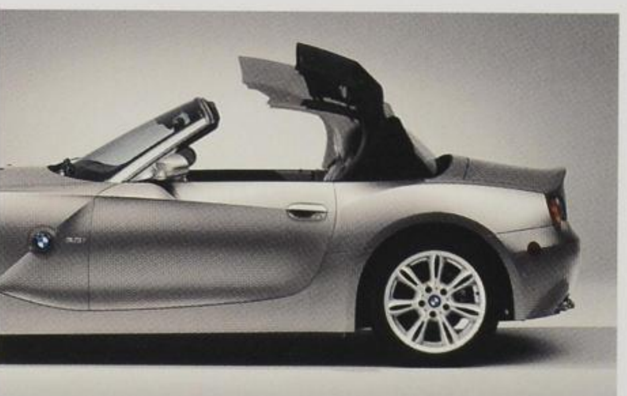
□ Fully automatic, lined power softtop is completely automated. To open or close it, press a button at the front of the center console. The top automatically unlatches from the header and folds down neatly. An interior lining helps reduce wind noise and enhances insulation. Available in Black, Gray and Dark Beige.
