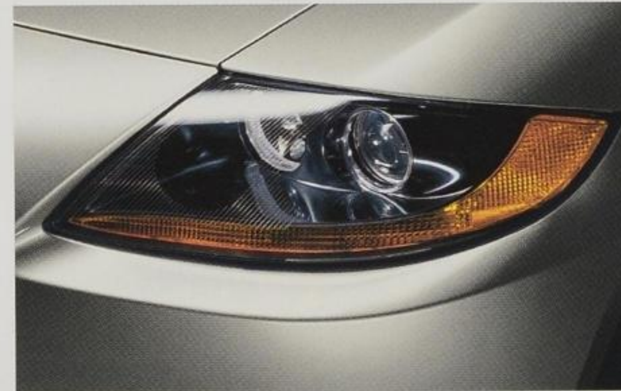
■ Halogen ellipsoid low-beam (outboard)/free-form high-beam (inboard) headlights are underscored by the sweep of amber turn-signal indicators and black high-gloss shadowline trim. (shown: Z4 2.5i with titanium-finish surround)
