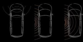
QuietTuning measures fall into three categories. First are those that reduce noise at its source – from the tread pattern of the tires to the damping of the engine mounts. Secondly, materials are used to block the noise path – from triple-sealed doors to an acoustic laminated windshield. Finally, noise is absorbed in the cabin with features like acoustic absorbers and specially designed carpeting.
