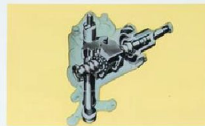
NEW MAGIC-CIRCLE STEERING . . . Ford's new recirculating-ball type steering mechanism uses low-friction steel balls instead of usual worm gear. Magic-Circle Steering is designed to reduce steering effort whether driving or standing still.
