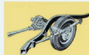
NEW, SMOOTHER RIDING REAR SUSPENSION . . . The springing action on the 58 Ford has been softened and shock absorbers newly valved for a smoother ride. Ford's new spring-leaf design means a better balanced, more uniform ride.
