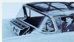
DOUBLE-WALL STEEL SAFETY DASH . . . This triple-insulated, double-walled protection between passenger area and engine compartment means greater quietness, a more durable, safer body.
