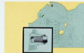
NEW SOFTER-ACTION BALL-JOINT FRONT SUSPENSION . . . The upper control arm pivots of Ford's new, smoother riding front suspension have exclusive Ford-designed threaded bushings that are permanently sealed and lubricated for longer life.
