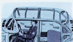
EXTRA-RIGID ROOF SUPPORTS AND BRACES . . . New fluted roof panel is supported by 5 all-steel roof cross braces. In addition to giving reinforcement to the roof, they provide valuable passenger protection in case of roll-over.
