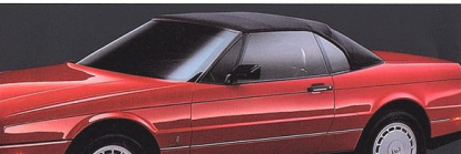
Allanté's power-latching soft-top design features gas-strut assist, electrically heated glass rear window and glass quarter windows
