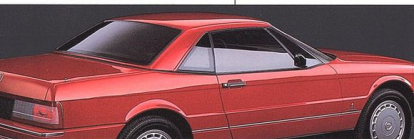
The aluminum hardtop weighs only 58 lbs., and fastens quickly into place. Includes heated rear window and glass quarter windows
