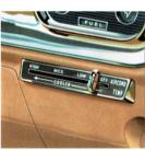
The Cadillac Air Conditioner for 1957 has been completely redesigned. Located completely forward of the passenger area, it circulates outside air that has been filtered of dust and pollen and has been cooled to the temperature the driver desires. It is available as actra-cost item on all models.
