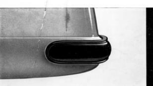
REAR END PROTECTION. Rubber-faced bumperettes curve right around the vital rear corners, absorb shocks better and do not show scratches.
