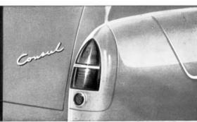
compact twin tall-light assembly . . . incorporates red stop light, amber flashing turn-indicator lights and built-in reflectors.
