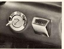
A handbrake warning light alerts the Fairmont driver when the handbrake is on, as he goes to drive away.
