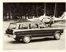
The Fairmont Station Wagon features the electric tailgate window which can be operated by pressing a switch from the driver's seat, or turning the key in the tailgate.
