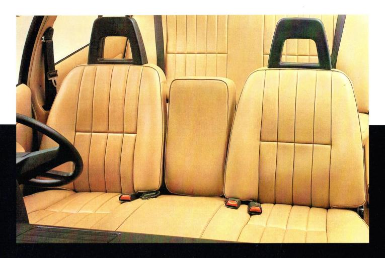
To provide legroom for the centre front seat passenger, Centafold will only be fitted when ordered in conjunction with a column shift automatic or manual transmission and a centre console will not be installed.
