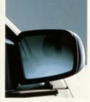
4. Meteor Ghia offers electrically operated left and right hand exterior rear view mirrors. On the GL there's a manual remote control mechanism for the driver's side exterior mirror.
