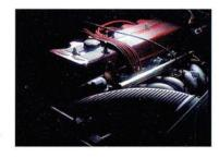
the 4.0 litre Ford multipoint EFI six cylinder engine.
