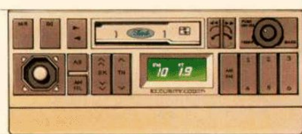
The radio and cassette player is protected by a programmed security code rendering the unit useless to thieves.
