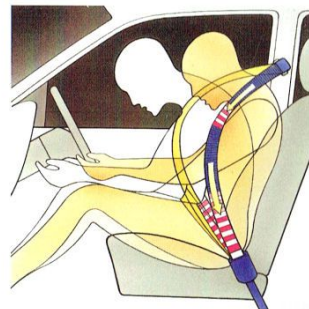
Belt-locker device instantly prevents payout of seat belt webbing.
