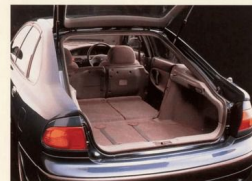
TX-5 Ghia demonstrates its versatility with a 60/40 split rear seat that offers a variety of passenger and luggage area combinations. Lower the short side (top) and there's space for extra cargo but still with room for two rear seat passengers. The other side of the rear seat lowered (middle) gives more luggage area and allows one passenger in the back. Or (bottom) lower both sides to open up a cavernous cargo area.
