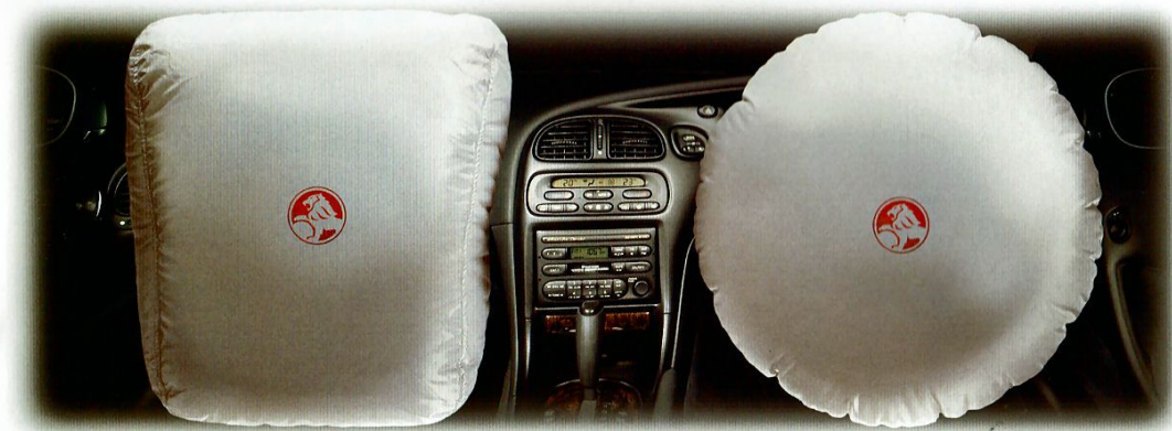
Calais airbag system The Holden Calais features a driver and front passenger airbag system as standard equipment. These deploy simultaneously in milliseconds in conjunction with the front seat belt pre-tensioners. They also use 'ladder' technology to help prevent aggressive airbag injuries.
