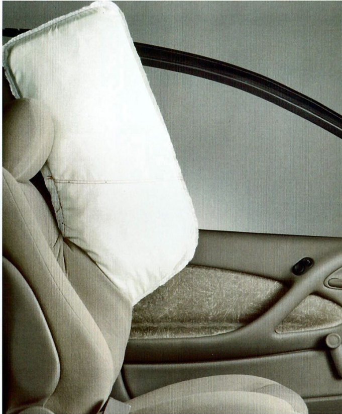
First Australian built car with Side Impact Airbags* Deploying within milliseconds at 45° away from the occupant, Calais' side impact airbags will be in optimum position regardless of seat angle.
