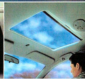
The HBD tailored sunroof is electronically controlled from convenient ceiling mounted controls for preferred positioning in the slide or tilt mode, and even automatically closes when you lock your car.
