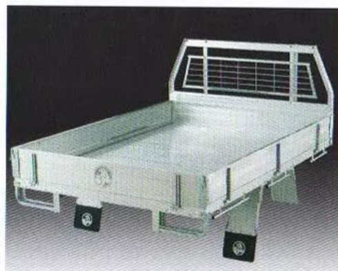
Generic Alloy Tray: Features general purpose or (optional) heavy duty aluminium floor, standard 225mm alloy dropsides, quick hitch rope rails, tapered headboard, rear window protector and Holden branded mudflaps
