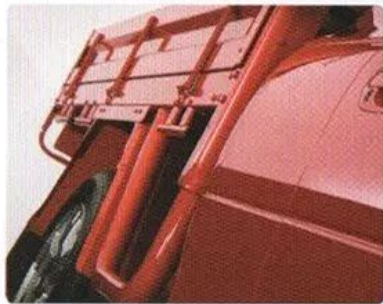
Practical, good looking stirrups incorporated into the styled, tube headboard (available on enhanced trays only)
