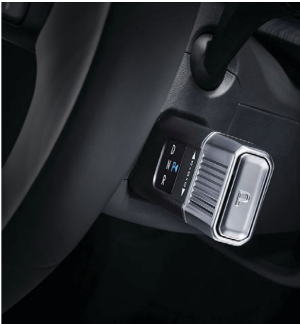
Shift-by-Wire gear selector
