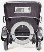
Here is shown the large clear-vision plate-glass window; the strong, double tyre carrier, accessible perrol tank and beautifully formed double crown mud guards.
