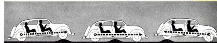
When the wheels of the Airflow Chrysler pass over a bump there is no pitching movement. Passengers literally float over it, due to relocating the pivoting points over the axles
