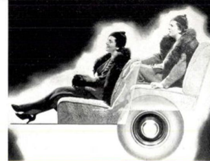
Rear seat passengers ride 20 inches in front of rear axle in the Airflow Chrysler, not over it
