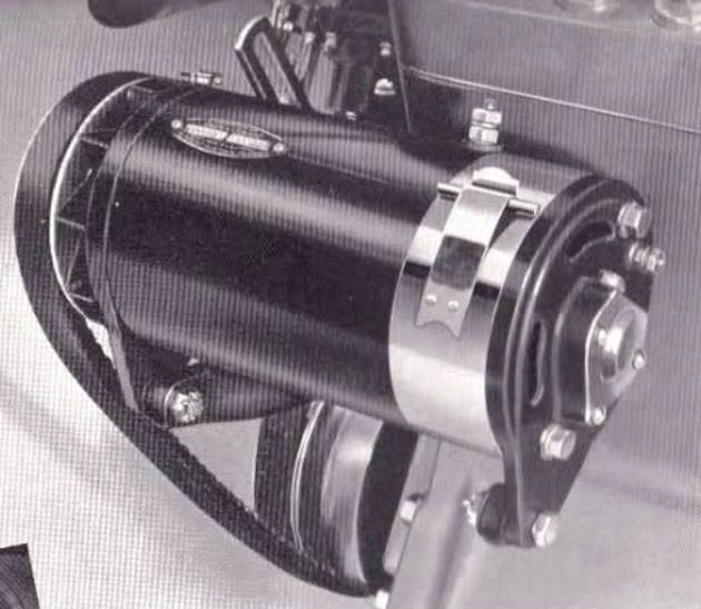
The new type of Semi-Centrifugal Single-Plate Clutch is shown at the left. Directly above is a view of the "Peak Load" Generator that automatically keeps your battery at its peak, regardless of radio, headlights or other withdrawals.
