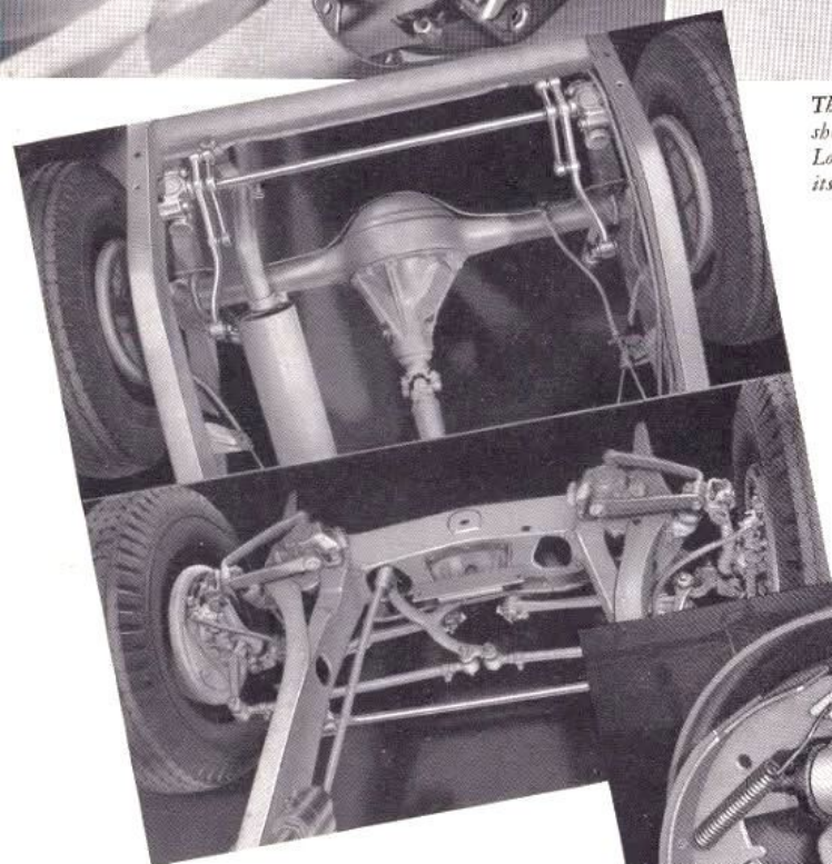
Cadillac's stabilizers, shown above, are stiff torsion rods that keep the car on a level keel when rounding curves or traveling on uneven roads. At the right is a view of the new hydraulic brakes. Always equalized; operate with minimum pedal effort. Important features: self-energizing action, weatherproof protection, protected fluid lines and double brake pistons.
