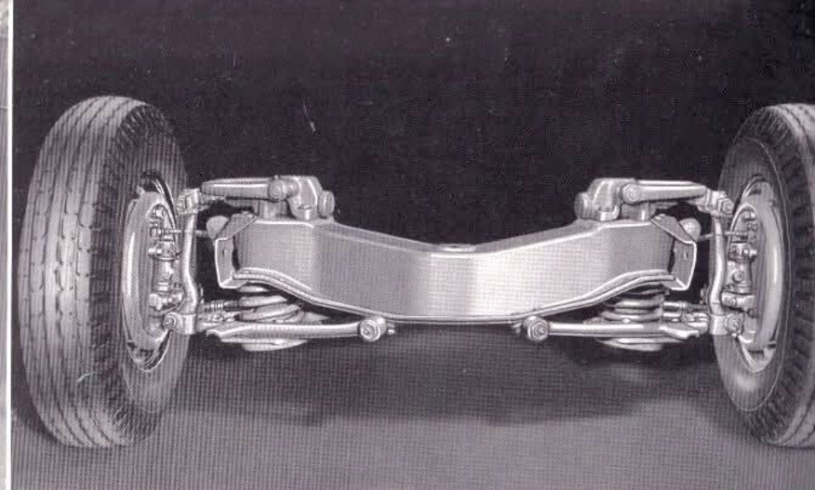
Above is pictured the mechanism of Cadillac's Knee-Action Wheels which contribute so largely to relaxed riding comfort on every kind of road and eliminate the pitch and bounce of the conventional rear seat ride. A truly marvelous feature.
