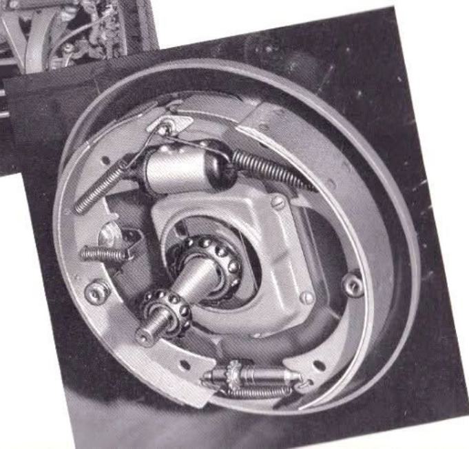
Cadillac's stabilizers, shown above, are stiff torsion rods that keep the car on a level keel when rounding curves or traveling on uneven roads. At the right is a view of the new hydraulic brakes. Always equalized; operate with minimum pedal effort. Important features: self-energizing action, weatherproof protection, protected fluid lines and double brake pistons.
