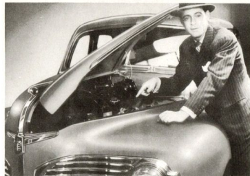
● Dodge Luxury Liner engines are easy to service through this wide-opening hood. The battery is under the hood in the fan blast where it will keep cool and where it is easy to check and fill. Less likely to be neglected.
