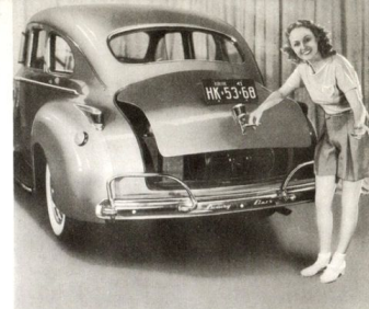
● The big, roomy luggage compartment has a spring counterbalanced lid that raises and lowers without effort. When open wide it stays open without a locking device. The spare wheel is mounted at the side for convenience in checking when compartment is full.
