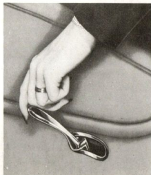
● Luxury Liner fittings include a convenient ash receiver on the instrument panel.
