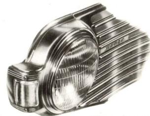
● The new sealed beam headlamps are an integral part of the grille design. Parking lights are at the side of the headlamp, and emphasize the width of the car.
