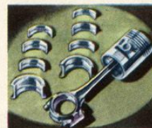
Piston rings are lower in the piston; removed from heat. Both pistons and rings are improved.
