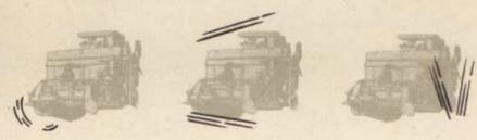
Engine mountings must permit some of this freedom of motion, yet hold the engine securely and prevent this motion from being noticed by the car's passengers.
