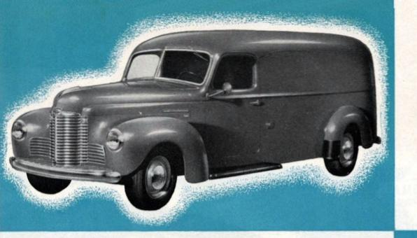
Handsome, large-capacity International streamlined de luxe panel bodies are rigidly constructed for safety and long life. The trim, symmetrical lines are further enhanced by the pressed-in belt and panel moldings. The panel body has a capacity of 171 cubic feet and measures 109 % inches long at the floor, 46 % inches between wheel housings and 56 inches high.
