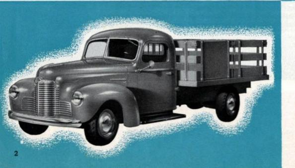
An 8-foot, light-duty, panelstake body with 14-gauge welded steel understructure and thoroughly seasoned oak floor is available for the 130inch wheelbase Model KB-3 chassis. The one-piece front section and the two-piece side sections are removable and are fitted to the top with interlocking connections. Inside measurements are 96 inches long, 78 inches wide and 30 inches high.
