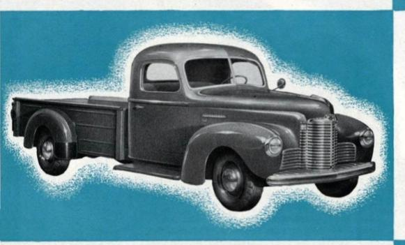
Pickup bodies have exceptionally large load capacities. The lines of the long all-steel drop-skirt bodies blend with the graceful contours of the grille head, cowl and cab, forming a light-duty transportation unit of distinctive appearance and maximum utility. Loading space is 102 inches long, 48½ inches wide and 17 inches high at the top of the 4-inchwide flareboards.
