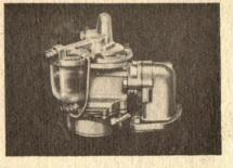
VACUUM BOOSTER PUMP—maintains high vacuum for constant speed operation of windshield wipers during acceleration or hill climbing. Assures clear vision always.
