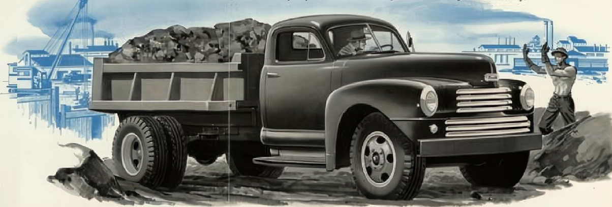
DUMP BODY —Mounted on Nash Chassis with 133-inch wheelbase. Expanded load carrying capacity and greater flexibility is gained with a two-speed rear axle available on all models as optional equipment.
