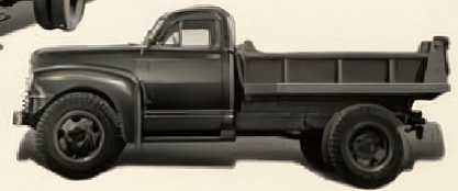
DUMP BODY —Mounted on Nash Chassis with 133-inch wheelbase. Expanded load carrying capacity and greater flexibility is gained with a two-speed rear axle available on all models as optional equipment.
