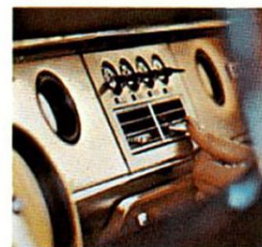
Toggle switches control instrument panel courtesy lights, rear roof pillar courtesy lights and dual map lights mounted in Overhead Console.
