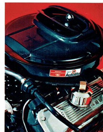
CJ 428 Ram V-8 features air induction hood scoop to give your Cougar extra muscle, and aluminum rocker arm covers.
